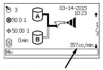
Fig. 63. Status Screen Flow Rate Display
